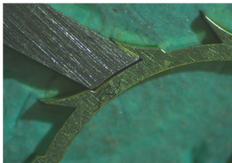
The fit of the tooth-straightening rig, under magnification – picture courtesy West Dean College
